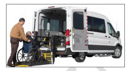
BODY ON CHASSIS VEHICLE WITH LIFT (13- TO 21-PASSENGER; CAN BE CUSTOMIZED TO INCLUDE MORE WHEELCHAIR TIEDOWNS AND REDUCE OVERALL PASSENGER COUNT)
